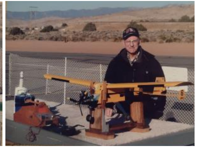
Harold Siegfried's Swizzle Stik. Note the sub rudders on the horizontal stab
