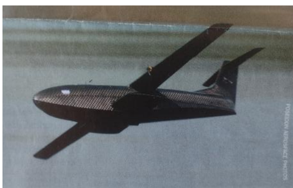
The 13-ft.-span, electric-powered Seagull subscale model has conducted flight tests.
