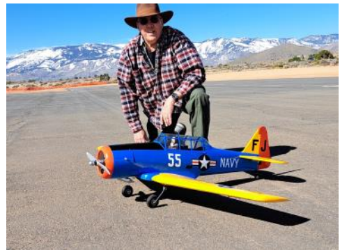
Larry's AT6 Texan Maiden flight Mar. 21, 2024 Wing span 67.5 inches Weight 7.8 lbs Motor OS 91 4 stroke surplus Propeller 14x6 Hanger 9
